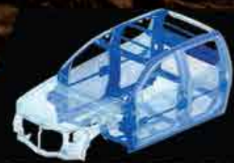
The cabin is constructed from high tensile tailor blank welded steel for unyielding strength and rigidity of the passenger safety cell
