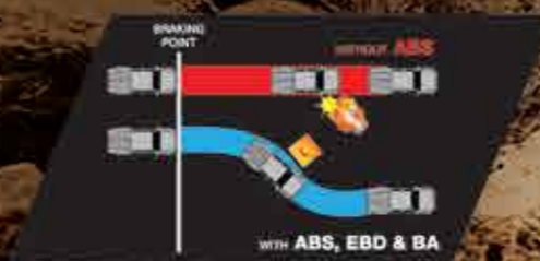
Optimum Steering Control, when brakes are applied, with Anti-Lock Braking System (ABS), Electronic Brake-Force Distribution (EBD) and Brake-Assist (BA)
