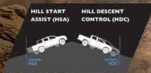
HSA prevents rollback on gradients above 5.7 degrees, while HDC provides maximum traction going downhill
