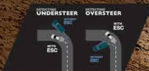
Included on all D-MAX V-Cross models, Electronic Stability Control (ESC) detects if the vehicle is under or over steering
