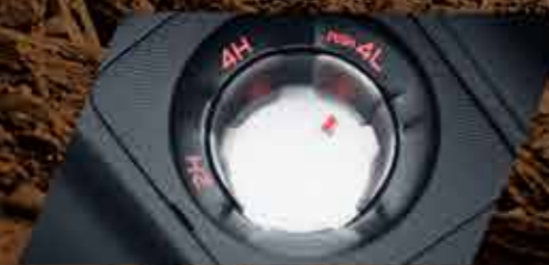
"Terrain Command" 4WD system allows for simple shift from 2WD-high, 4WD-high and 4WD-low
